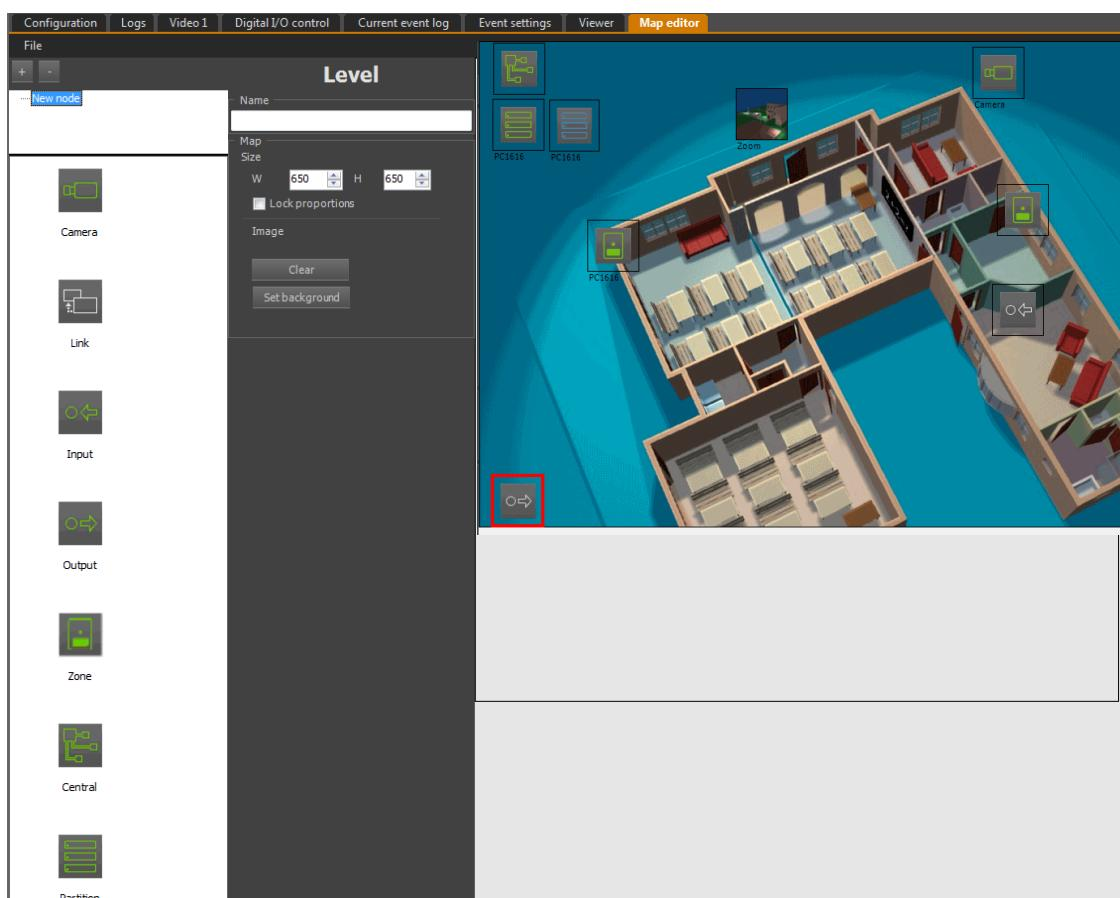
After placing the element icons on the map, define their parameters. To do this, click each icon in the design area one by one and edit the following parameters:
