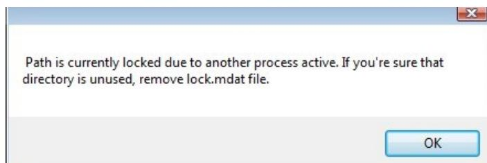
In this case, remove the lock.mdat file from each folder for which this message appears.
