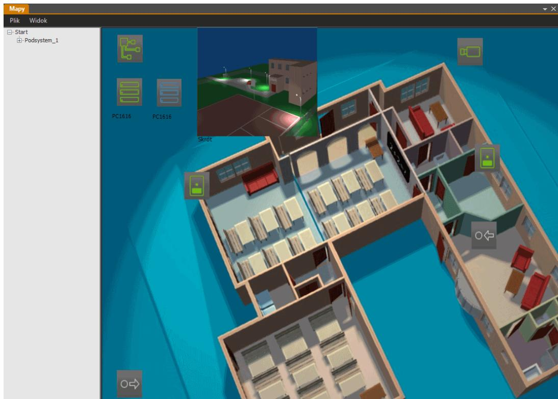
To change the currently displayed map, select File / Open in the preview window menu and load any map. In the View menu of the preview window, you can hide the map tree display with the Display tree option and lock the map's size proportions using the Lock aspect ratio.
