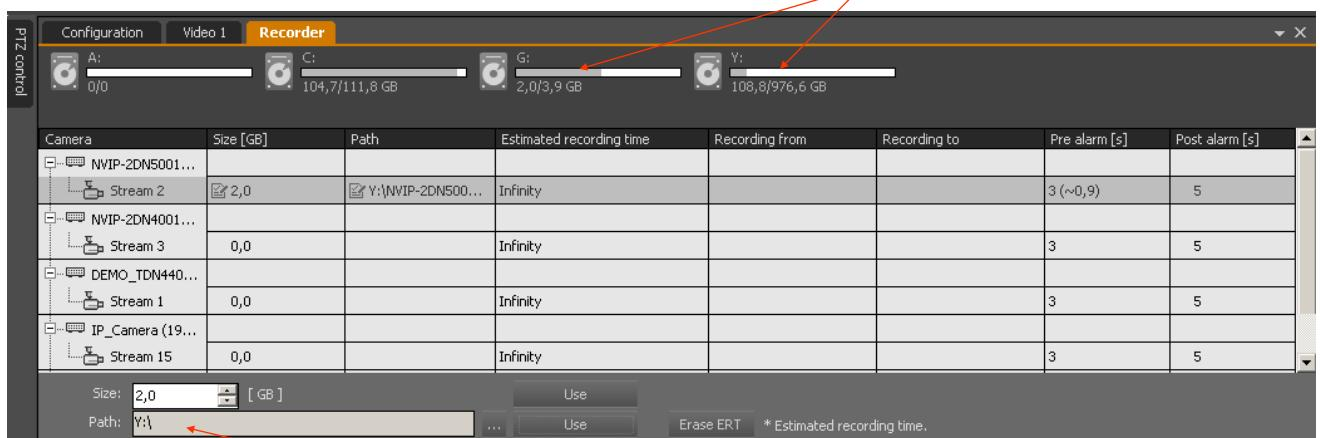
The assist bar allows you to enter a specific size and paths to all selected cameras simultaneously.
