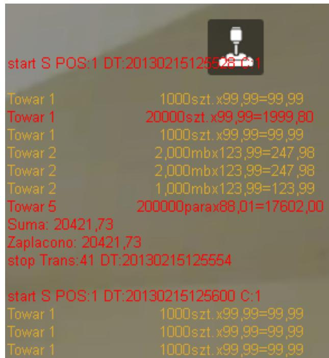
Lines containing the strings specified in the Highlighted text field are displayed in red (in the example above, the lines contain the string "20").
