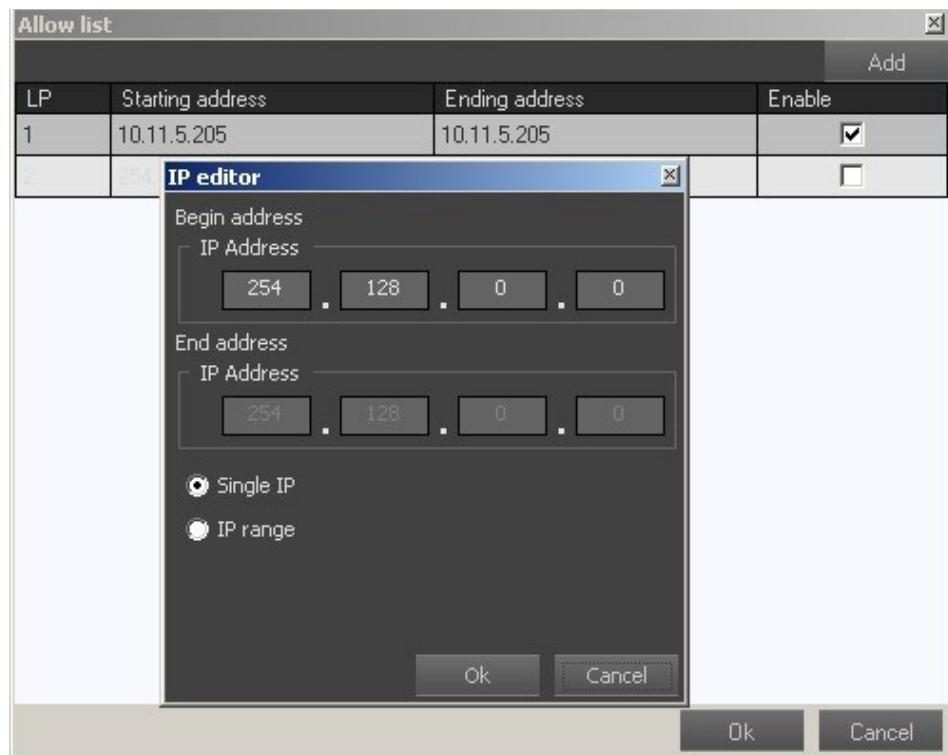
The Add button allows you to enter a range or a single IP address to the current list. To delete the selected IP address, right-click on it and select the Delete option.
