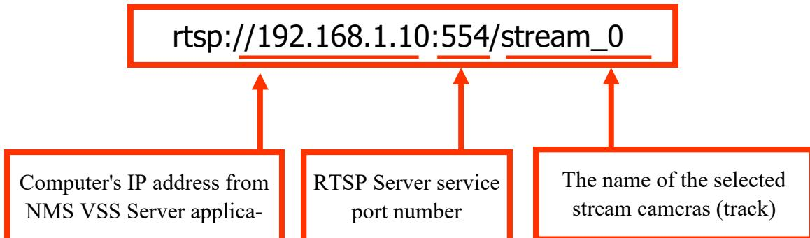
After correctly entering the network path and loading the player buffer, the image from the camera will be displayed on the screen.
