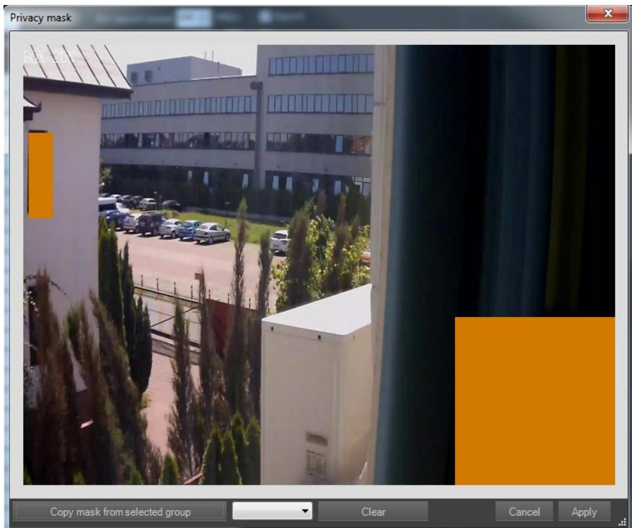
Selecting a part of the window with the left mouse button creates a rectangle masking the image. Pressing the right mouse button when the cursor is in the field will delete the mask. Selecting a window fragment with the right mouse button deletes all privacy masks that are in the selected field.
