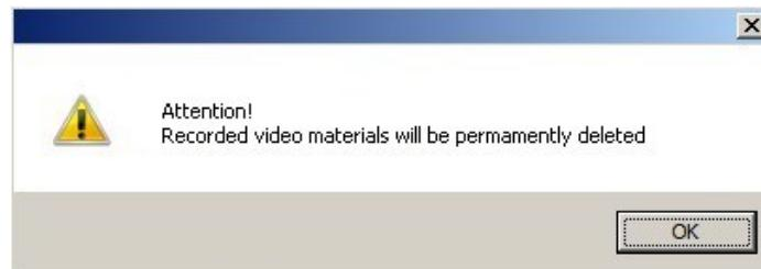
In order to completely delete recordings from a given camera, select the appropriate camera and select the Delete recording option from the pop-up menu or enter "0" in the camera size column and then click the Save button. Changing the path for existing recordings will also delete the recorded material for that camera. In both cases an appropriate message will be displayed.
