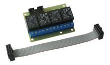
Device Type Description Normal load current AC1 category Normal load current DC1 category Relay board 10 A Relay board increases the functionality of the network I/O module V-1000/IOM with 4 additional relays 10 A / 240 VAC 15 A / 24 VDC
